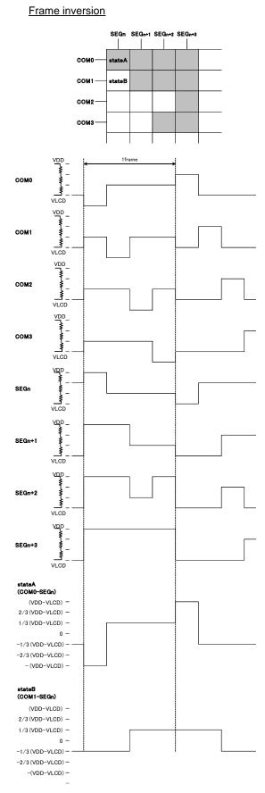
Figure 17. LCD waveform at frame inversion (1/3bias)
