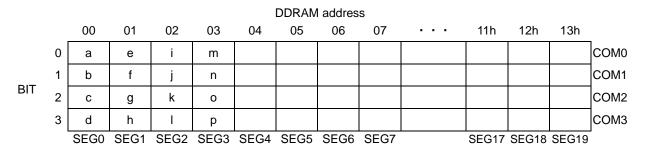
Data transfer to DDRAM happens every 4bit data. So it will be finished to transfer with no need to wait ACK.
