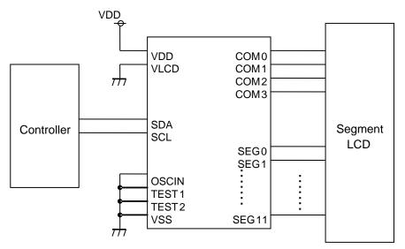
Internal Oscillator circuit use mode
