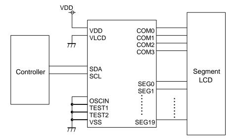
Internal Oscillator circuit use mode
