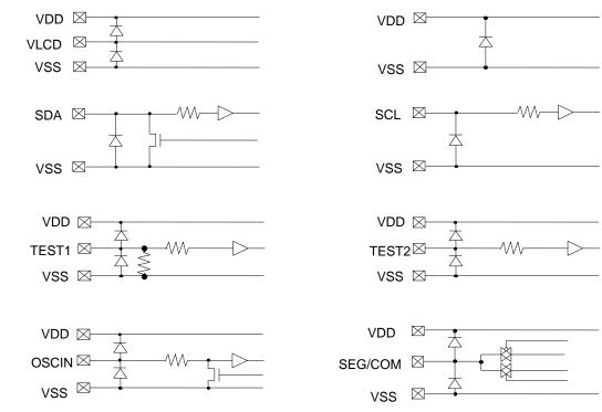
Figure7. I/O equivalent circuit
