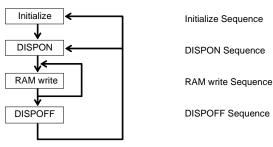
This LSI is initialized with Initialize Sequence. And start to display with DISPON Sequence. This LSI will update display data with RAM write Sequence.
