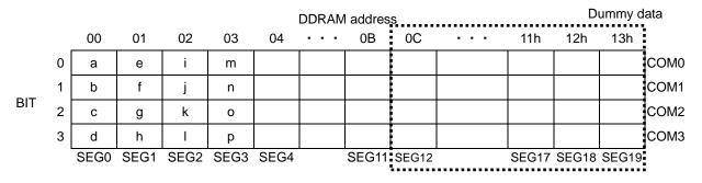
Data transfer to DDRAM happens every 4bit data. So it will be finished to transfer with no need to wait ACK.
